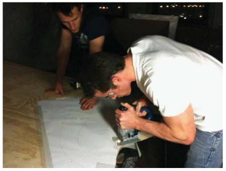
cutting wind support discs with plotted template
