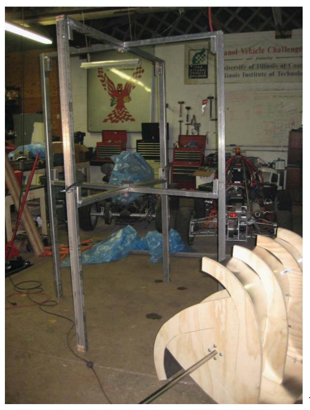
Savoius-Rotor wind turbine with completed frame
