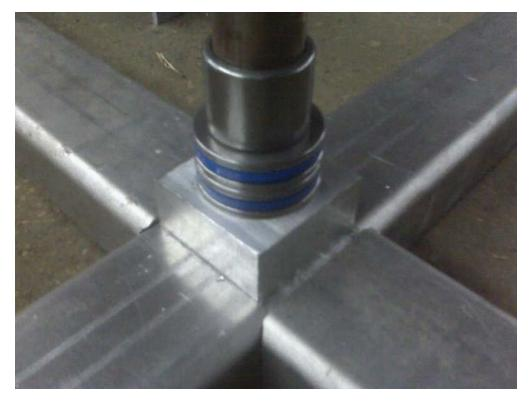
horizontal corss members with axial support block and ball bearings
