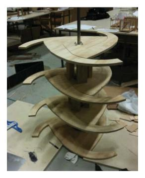
dry assembly of prototypical wind turbine
