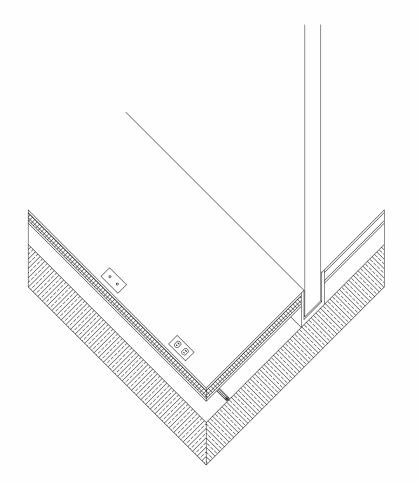
The collaboratory space levels have a raised loor that allows electric and data lines to run underneath the loor, leaving the space free to move the panels.
