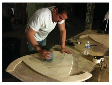
sanding wind support discs to reduce wind drag
