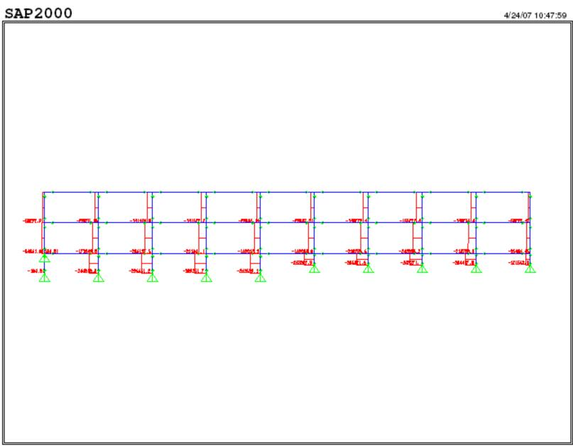
SAP2000 v10.0.7 - File:model5 - Axial Force Diagram (1.2D+1.6L+0.5S) - lb, ft, F Units
