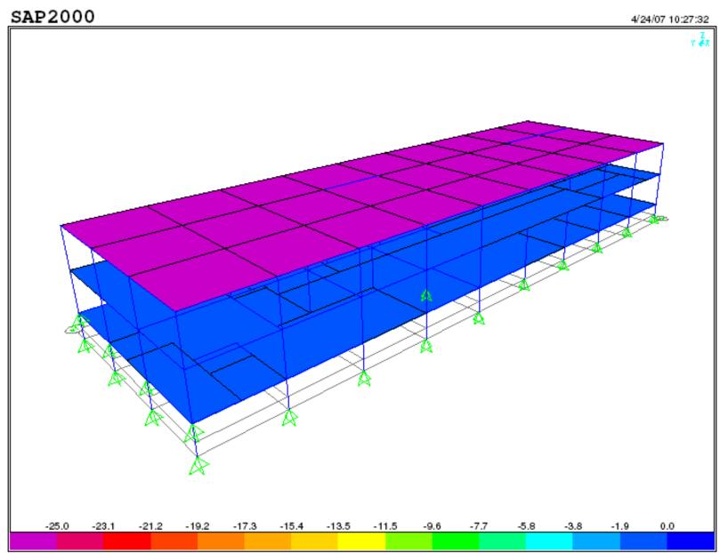
SAP2000 v10.0.7 - File:model8 - Area Uniform to Frame (Snow) (GLOBAL - Gravity) (2-Way) - Ib, ft, F Units
