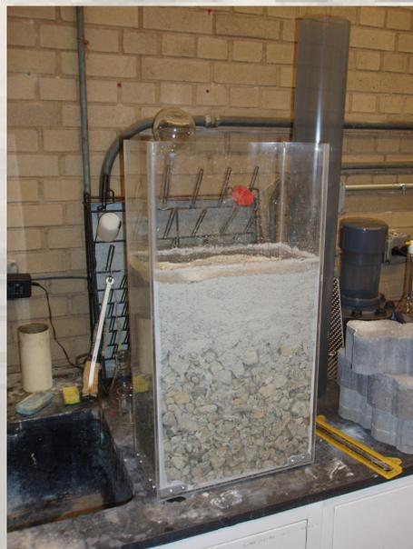
System in which polymer is placed directly in the gravel in a porous pavement system.
