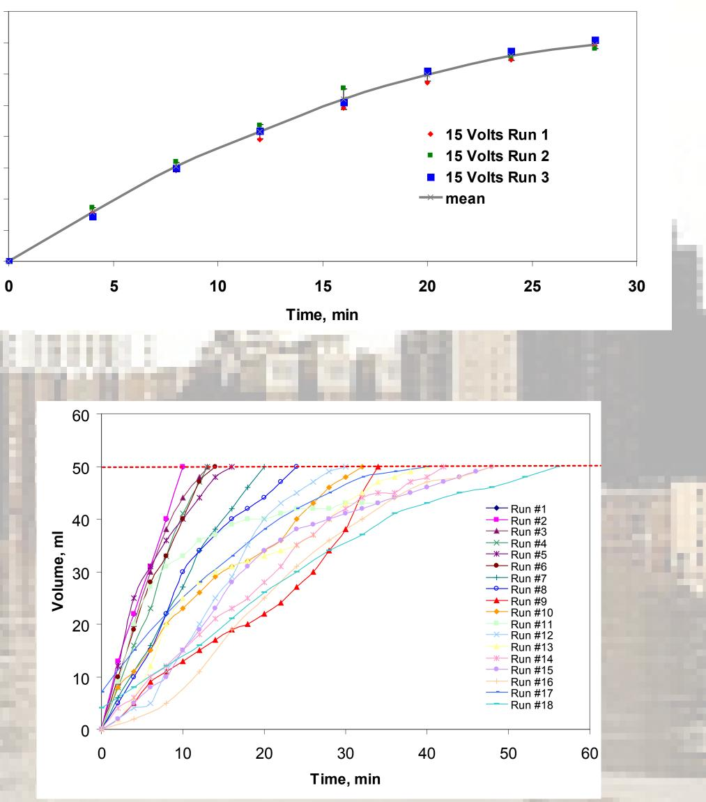
The polymer slowly deteriorates over multiple swelling and deswelling cycles.
