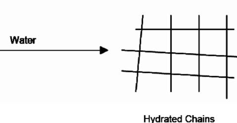
Polymer is basically a bundled net that stretches out when the polymer swells.
