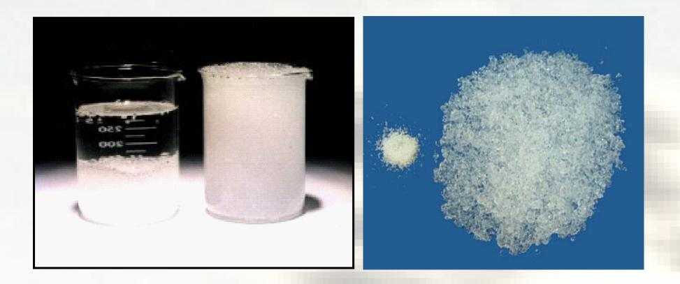
Super absorbent polymers (SAPs) are cross-linked polyelectrolyte materials that hold at least 100 times their weight of water.
