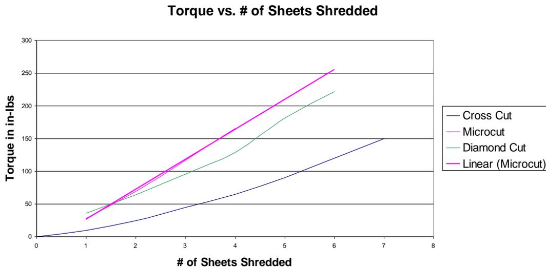
From the data above, diamond cut offered the best balance between security and torque required. Also, diamond cut and Microcut are rated at level 3 security while cross-cut is rated at level 2.
