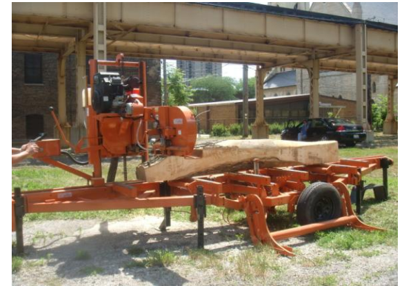
Portable Mill on site.
