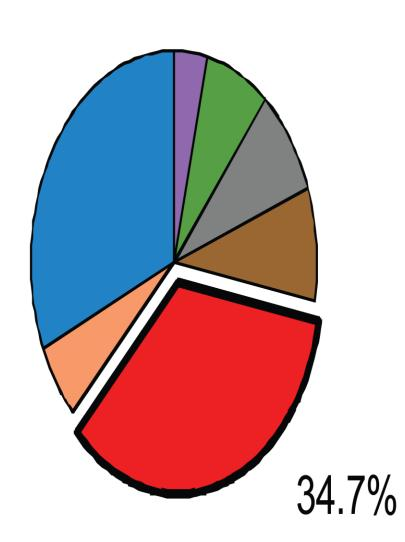
Percentage of pipeline accidents caused by excavation damage
