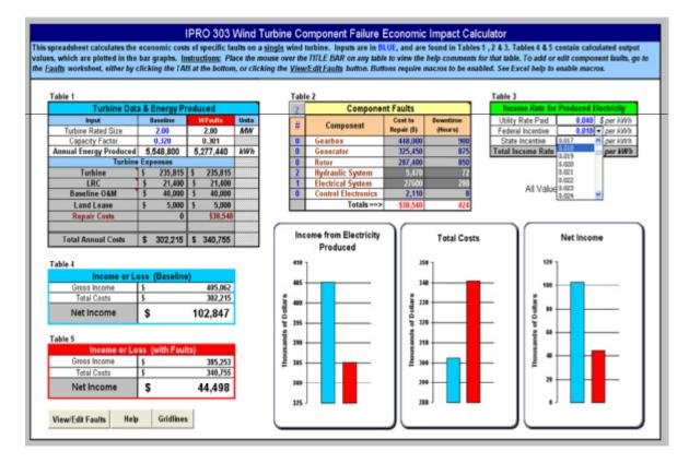
The second sheet from the workbook deals with specific faults in the wind turbine. The default sheet contains six common faults. The downtime, labor rates, equipment rental rates, and spare part costs are entered by the user. The spreadsheet then calculates total costs and down-time associated with each fault and populates a table. This table (table 2 in the main spreadsheet) is then used to calculate outputs. A screenshot of the faults spreadsheet is given below:
