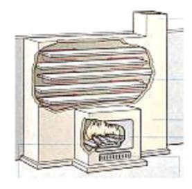
fireplace/stove connected to a cavity wall generates heat within the wall and creates radiant heating for the bedrooms at night when the temperature is the coldest, and will also heat the wall when the stove is in use.
