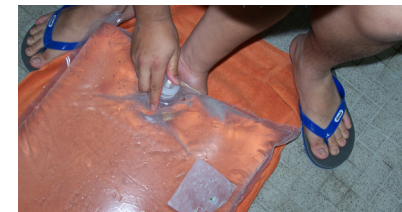
ACARA 1 testing a water storage bag prototype made from a 5 gallon milk bag.
