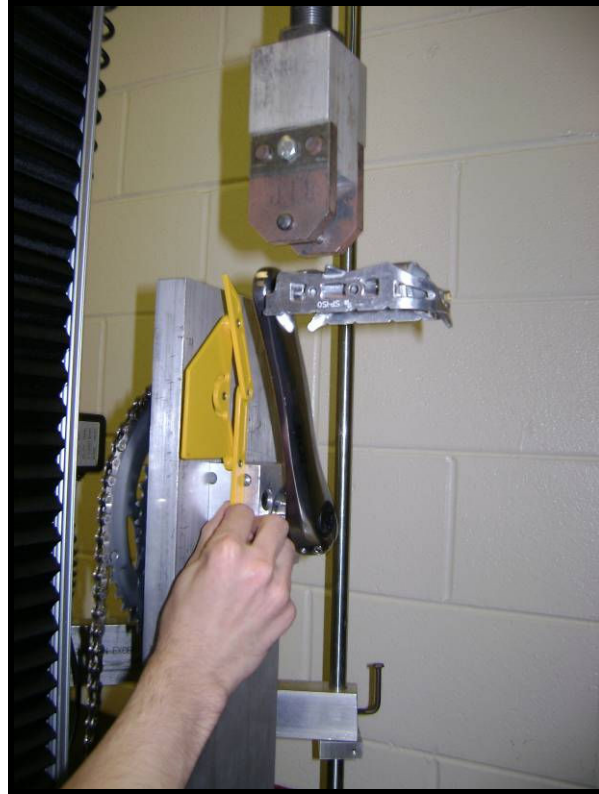
Figure 3. Measurement of angle before load is applied by the Instron 5500.
