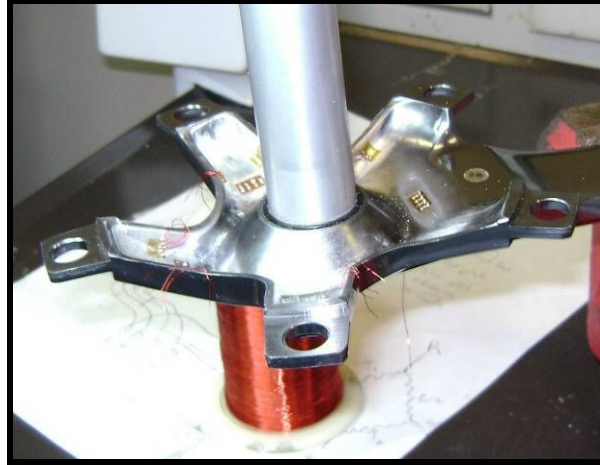
Figure 1. Placement of strain gages inside spider.
