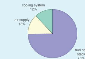
fuel cell stack cost- 80 kW direct hydrogen
