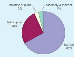
fuel cell subsystem - 80 kW direct hydrogen
