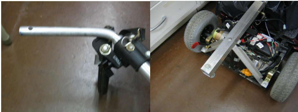
Figure 12: Ball-hitch for connection between vehicle and trailer
