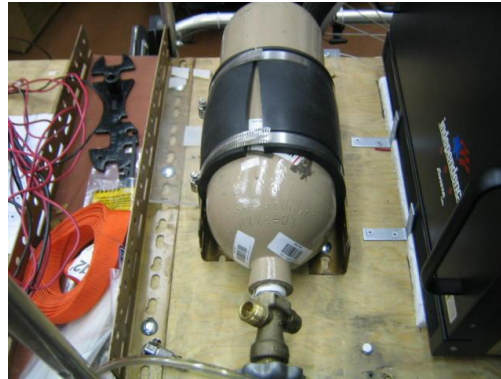
Figure 13: Hydrogen Tank Attachments
