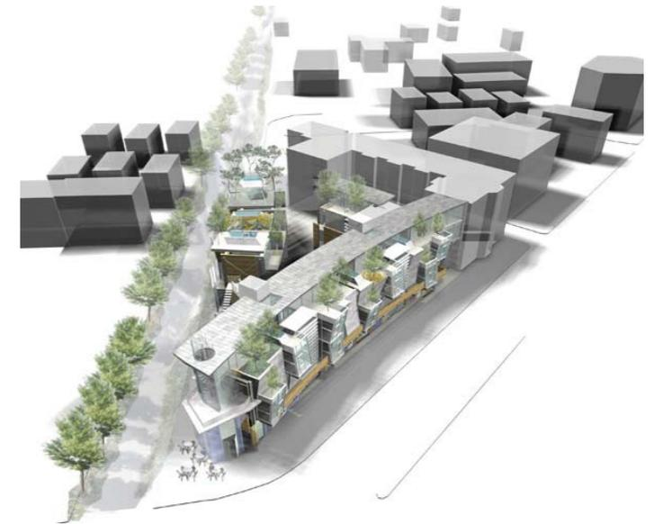
From Highway to Housing: What happens to the millions of tons of discarded materials from obsolete infrastructures like Boston's Big Dig? Destroying it costs millions to tax payers as well as wastes the embodied energy already stored in the materials. Dismantled and relocated, concrete and steel sections can become structural building modules adaptable to a variety of sites and programs.
