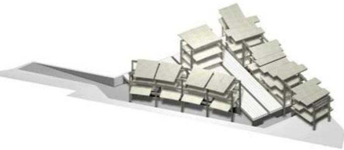
6. Lighter roof structures are connected to invert sets & vertical circulation is installed.
