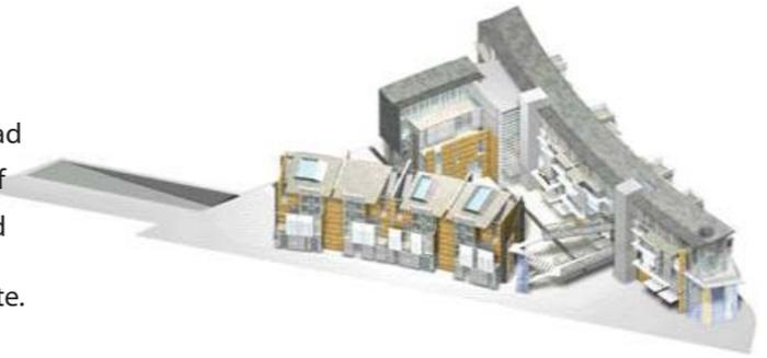
Cross section: The assembly of infrastructural materials provides advantages such as long span underground parking, the integration of water filled trombe walls, and the ability to incorporate full scale landscapes on roofs and balconies.
