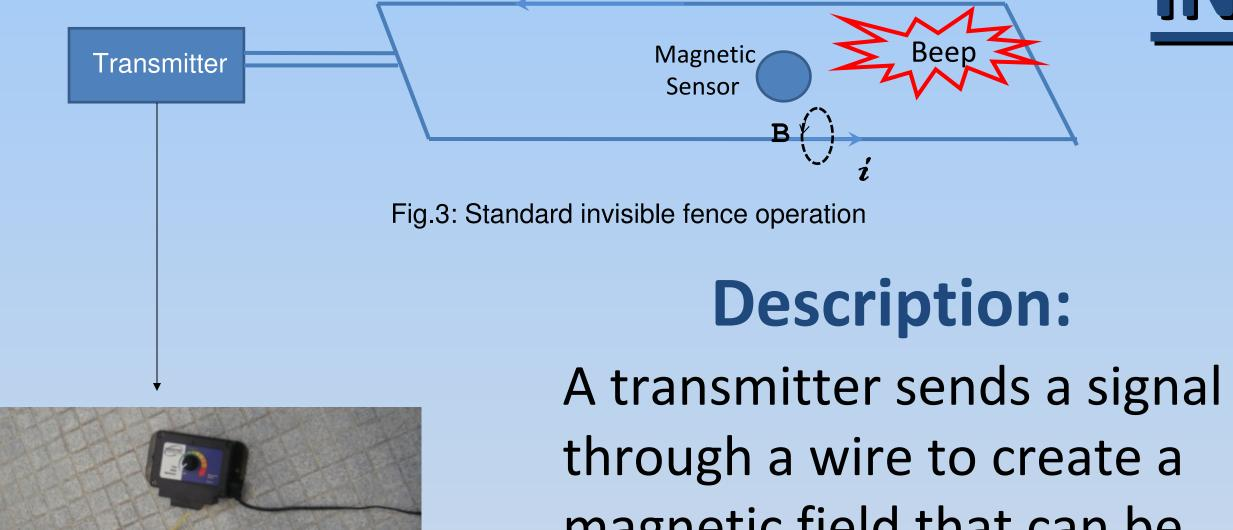
magnetic field that can be detected by a concealed receiver.
