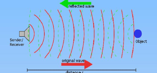
Fig.1: Standard SONAR operation
