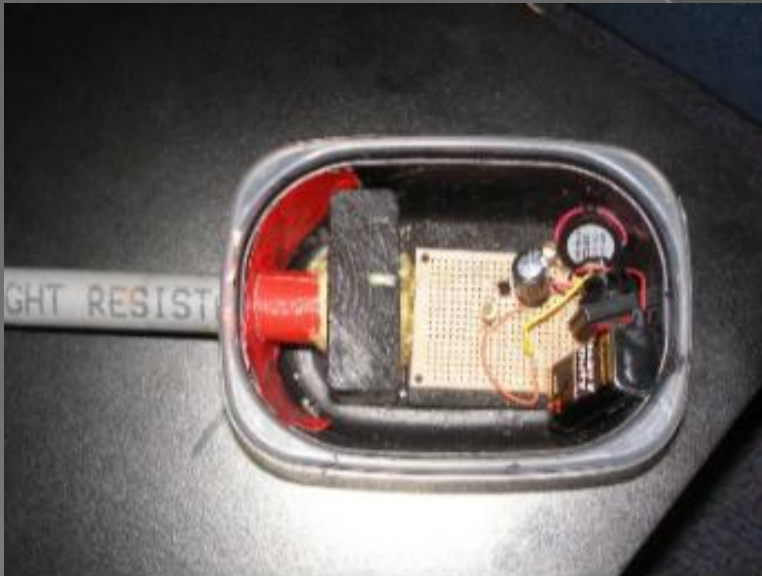
Prototype laser detector with lid off.
