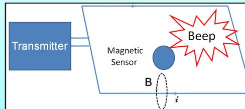
When the magnetic sensor approaches a certain distance from the wire, it gives off an alarm.
