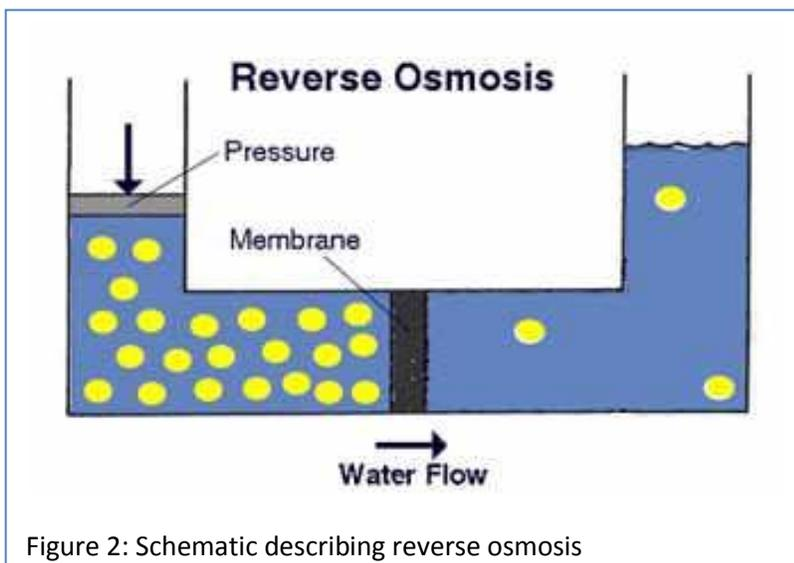
Figure 2: Schematic describing reverse osmosis
