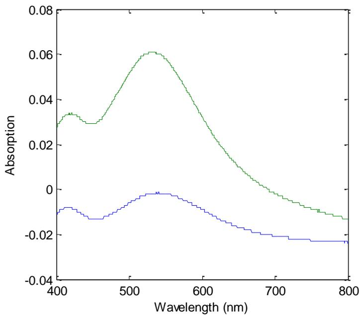
Figure 7: Nanorod Formation at 0.045 mL Seed Solution and 25°C
