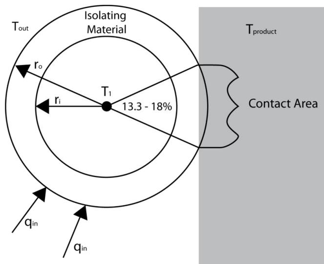
Figure 5: Heat Transfer Schematic for Silver Nanorod Thermal Indicator Label
