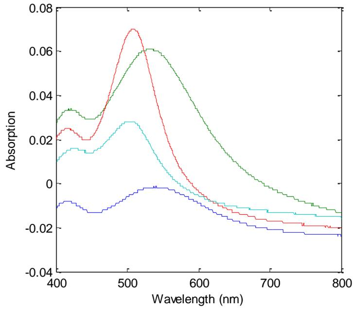
Figure 8: Nanorod Formation at 5 M NaOH and 25°C
