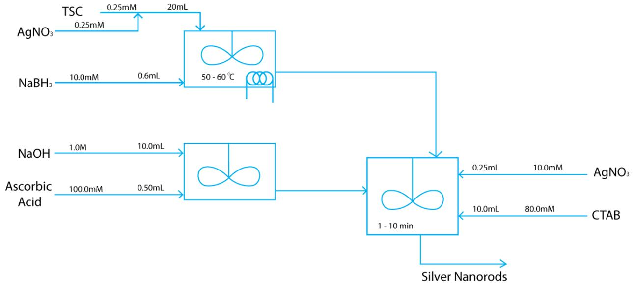
Figure 1: Silver Nanorod Production Process Flow Diagram
