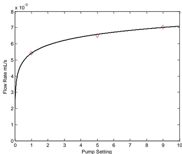
**Figure 4: Product Pump Calibration**
