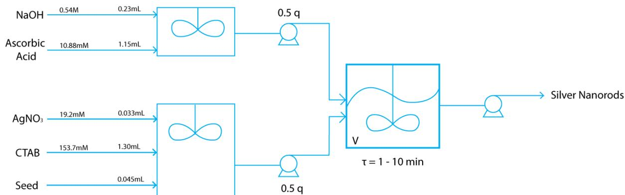
**Figure 3: CSTR Synthesis Process**
