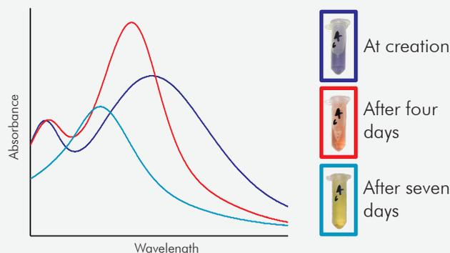
This graph shows a nanorod sample tested at three times: shortly after it was first mixed and centrifuged on the fourth day, and on the seventh day. The different peaks correspond to differences in physical shape.
