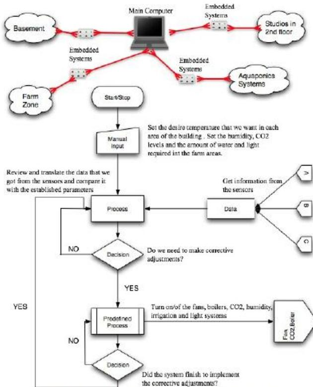
Figure 18. Control system architecture and flow control.
