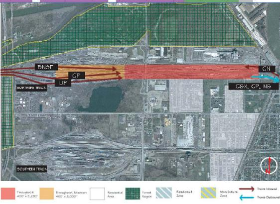
**Implementation-** The implementation of the Thruport system at the Riverdale rail yard. This layout uses the longest available length of track with room for expansion.
