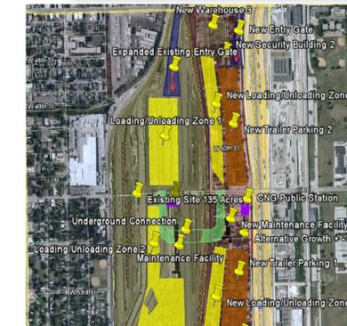
This team created a flipper model. A flipper is used to remove containers from trailers and improves the efficiency of the yards. Pictured on the left is the proposed layout of the intermodal yard, including a proposed expansion. This team also proposed a switch to compressed natural gas (CNG) as an alternative fuel, and a CNG station is included in this layout.
