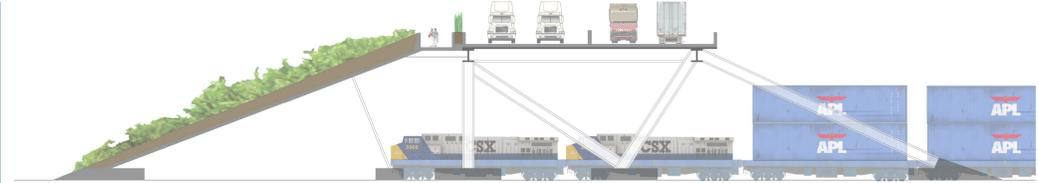
Cross section of bridge proposed by I PRO 307. The purpose of this bridges is to provide a safe path for cars, trucks, and civilians to cross the intermodal yard. On the bottom right is a proposed rezoning of the area, considering future development as well.
