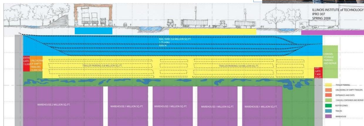
The graphic here provides a look at what goes on inside an intermodal yard. It shows a typical layout of the yard with color coding. The blue area represents the rails, and this is where containers are transferred from the trucks to the rail and the rail to the trucks. The yellow area is the trailer parking, where the trucks and containers are placed when they are not needed. The purple area are the warehouses.
