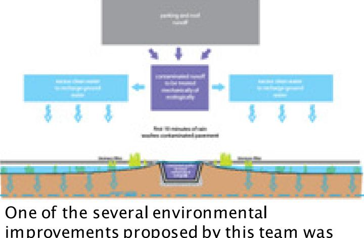
improvements proposed by this team was water retention. The diagram on top shows how runoff water is beneficial, and below how runoff will be collected in the yard.
