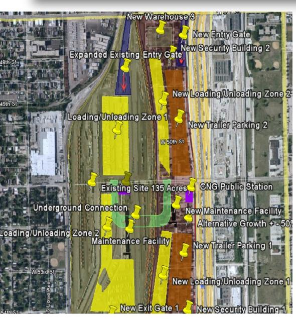
This team created a flipper model. A flipper is used to remove containers from trailers and improves the efficiency of the yards. Pictured on the left is the proposed layout of the intermodal yard, including a proposed expansion. This team also proposed a switch to compressed natural gas (CNG) as an alternative fuel, and a CNG station is included in this layout.
