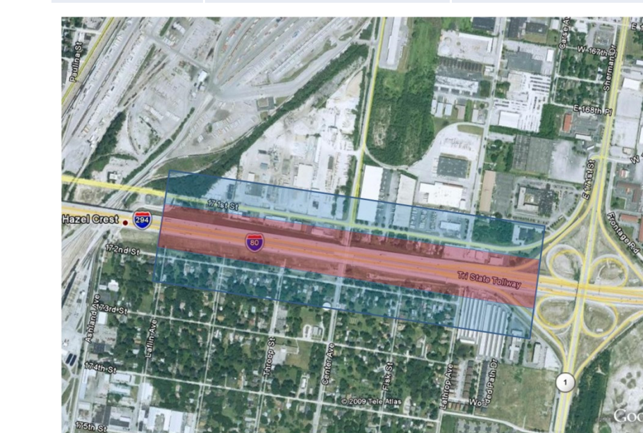
Image showing dBA range with the highway as a source. Red area is dBA>72. Blue area is less than 72 dBA and greater than 67 dBA
