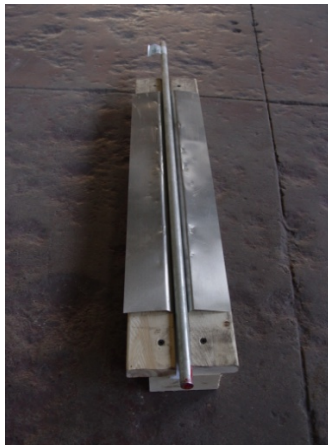
Bending of Sheet Aluminum to fit around copper pipe
