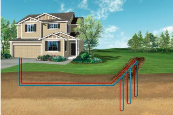
The ground is able to maintain a higher rate of temperature consistency because it absorbs 47% of the sun's energy (heat) as it hits the Earth's surface. Heat Pump geothermal systems are able to tap into this free energy with an earth loop. This technology is then used to provide your home or office with central heating and cooling.
