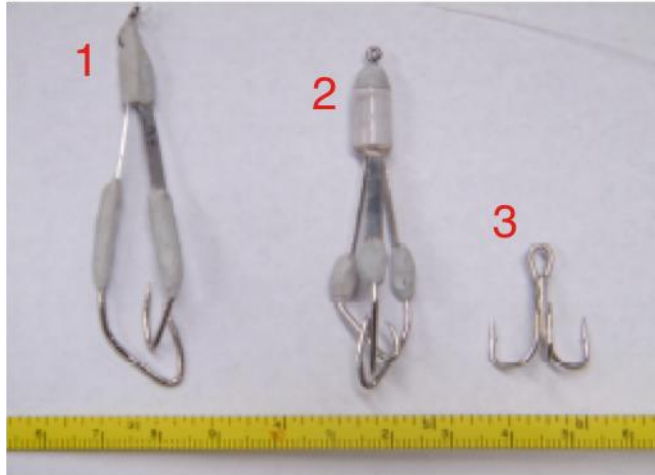
Figure 3. Mock-ups using epoxy to join the shanks and arms: Mock-ups 1 and 2 along with a traditional treble hook are shown. Mock-up 1 is a two-piece design, joined by epoxy; Mock-up 2 is a two-piece design with smaller epoxy joints. The third hook from the left is a treble hook; it is displayed for scaling purposes.
