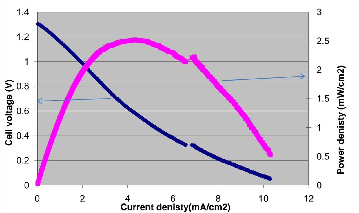
**Figure 3: Final polarization data from experimental results**
