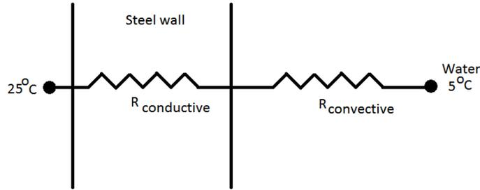
Figure 4 Heat transfer diagram.
