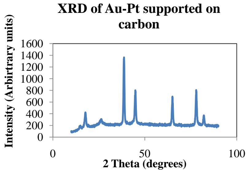
Figure 2: Lab results for second attempt at producing catalyst. This is a mixture of Au and Pt.
