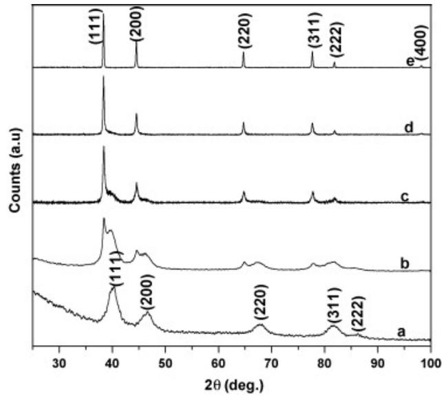
Figure 1: XRD data from literature; a is 100% Pt and e is 100% Au, b-d is mixtures of Au/Pt
