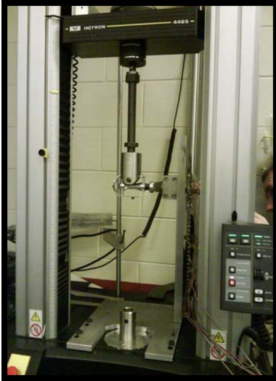
Figure R5: Test Stand in the Instron – Pulling
