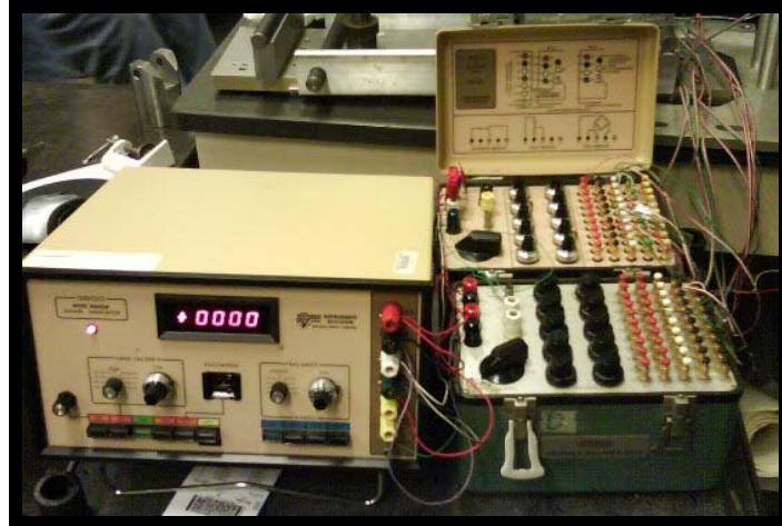
Figure R3: Switch and Balance Box with Strain Indicator
