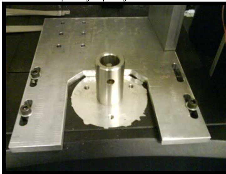
Figure R7: Base Plate for Test Stand Anchor
