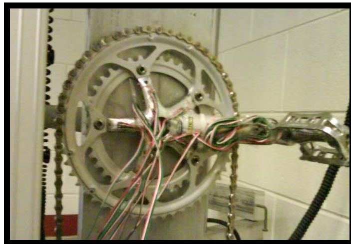
Figure R2: Placement of Soldering Tabs and Wires
