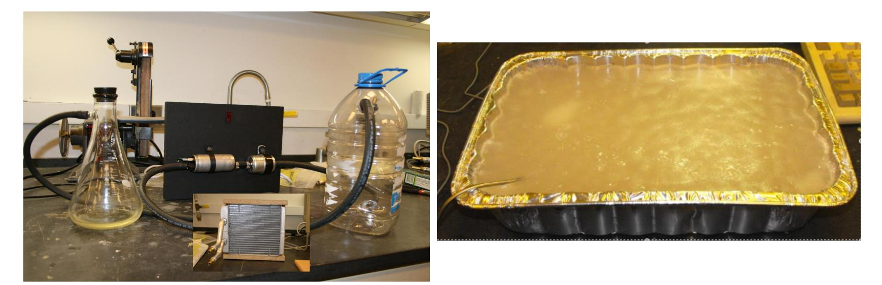
The refrigeration cycle prototype that has been designed by the team includes a fuel pump, reservoir tank, condenser, and a flask to heat the liquid.
