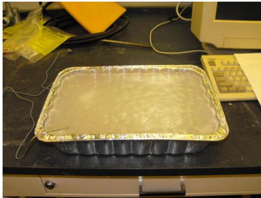
The water wall allowed cooling with no assistance, with ice packs, and with isopentane. The following results were obtained:
