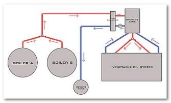
This image shows the vegetable oil system using two boilers in the Co-Gen facility. Waste heat is collected off of the boilers and carried through a heat exchanger. In the heat exchanger, heat is exchanged with another loop, which carries newly heated fluid into a storage tank. From this storage tank, it goes to the vegetable oil system just as the solar thermal fluid would.
