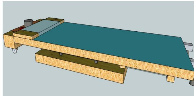
also a motor. The goal of this design is to automatically reach the correct frequency depending on the weight of the person, and shake the victim without the help from possible bystanders.
