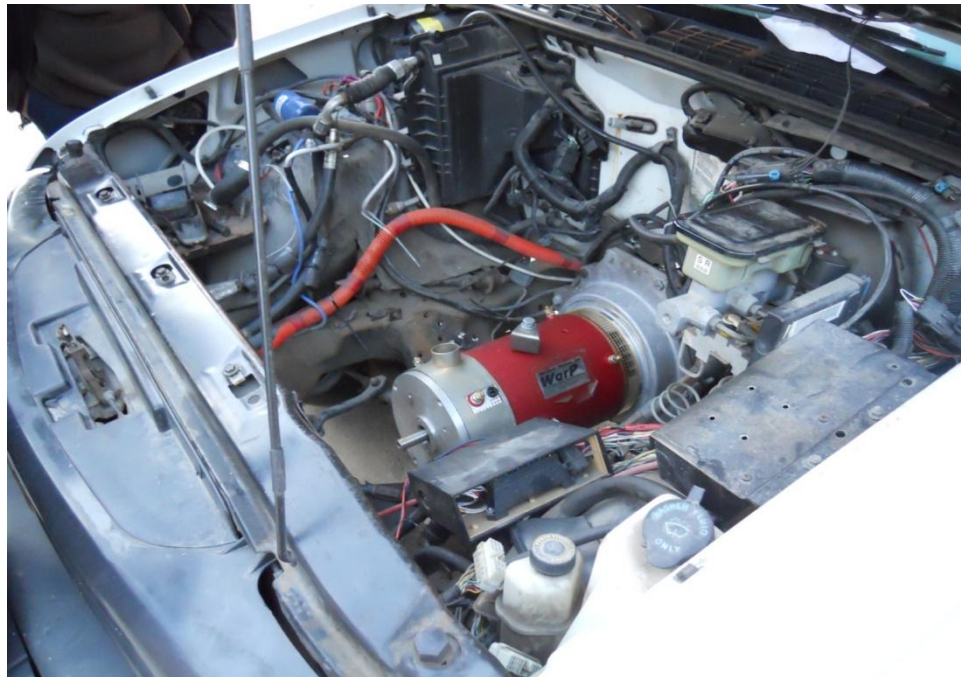
Figure 5: Installation of new electric engine and transmission.
