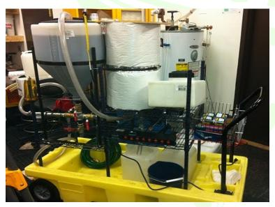
IIT facilities will need to find adequate space for the Microprocessor to be housed. The device itself is small, measuring roughly 5ft x 2ft x 5ft (*lwh*). The room were the microprocessor is housed needs to have a designated HVAC system for proper ventilation, since some of the chemicals used and produced are hazardous. Also, the room needs to have a blast door as well as a blast cabinet for methanol storage (Costs for these items can be found in the financial model below).
