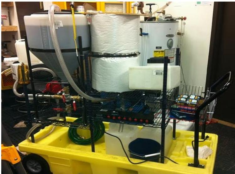
IIT facilities will need to find adequate space for the Microprocessor to be housed. The device itself is small, measuring roughly 5ft x 2ft x 5ft (*lwh*). The room where the microprocessor is housed needs to have a designated HVAC system for proper ventilation, since some of the chemicals used and produced are hazardous. Also, the room needs to have a blast door as well as a blast cabinet for methanol storage (Costs for these items can be found in the financial model below).
