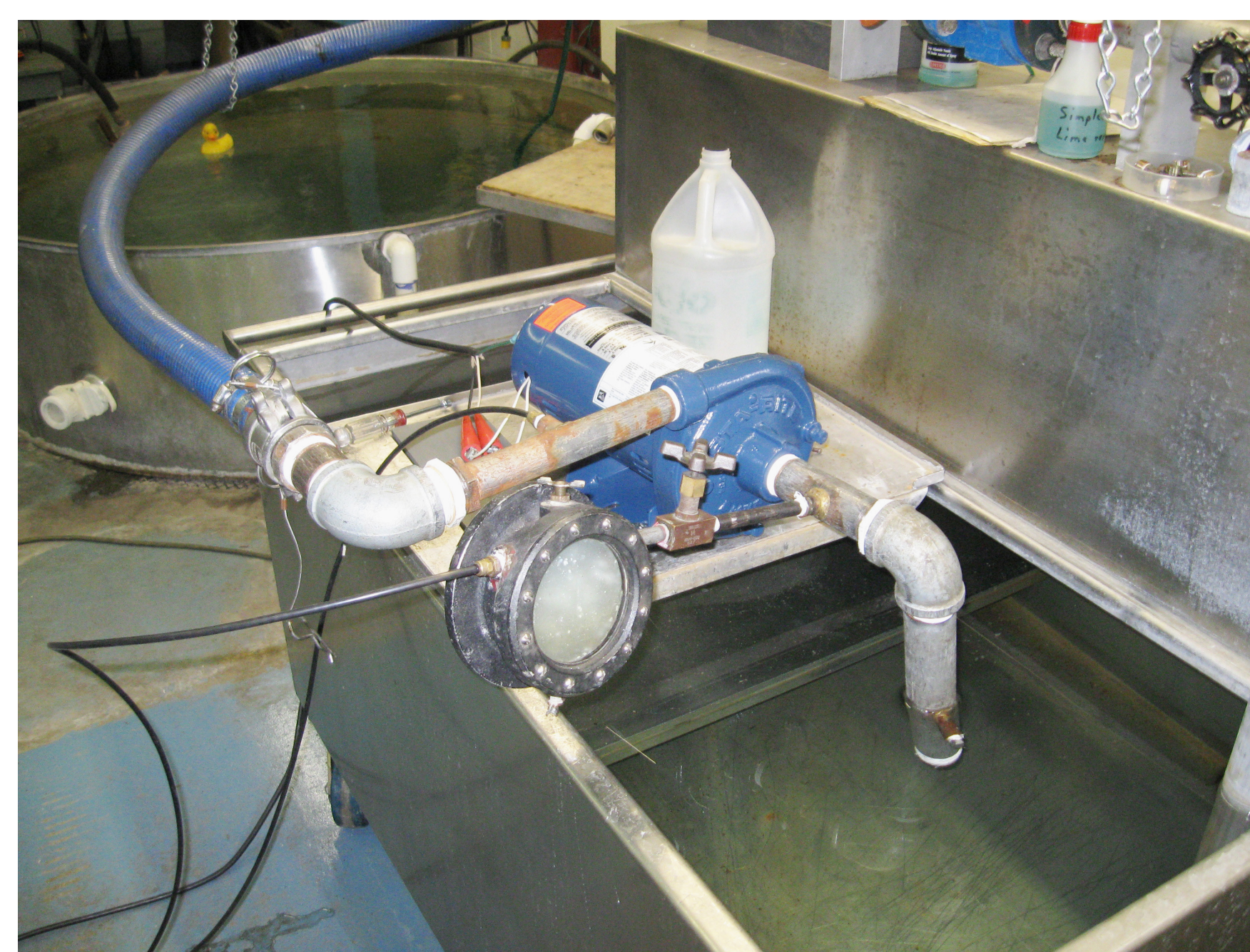
The pump testing station, with hoses leading to the differential pressure transmitters.
