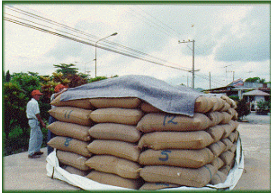
A properly stacked Cocoon before sealing
