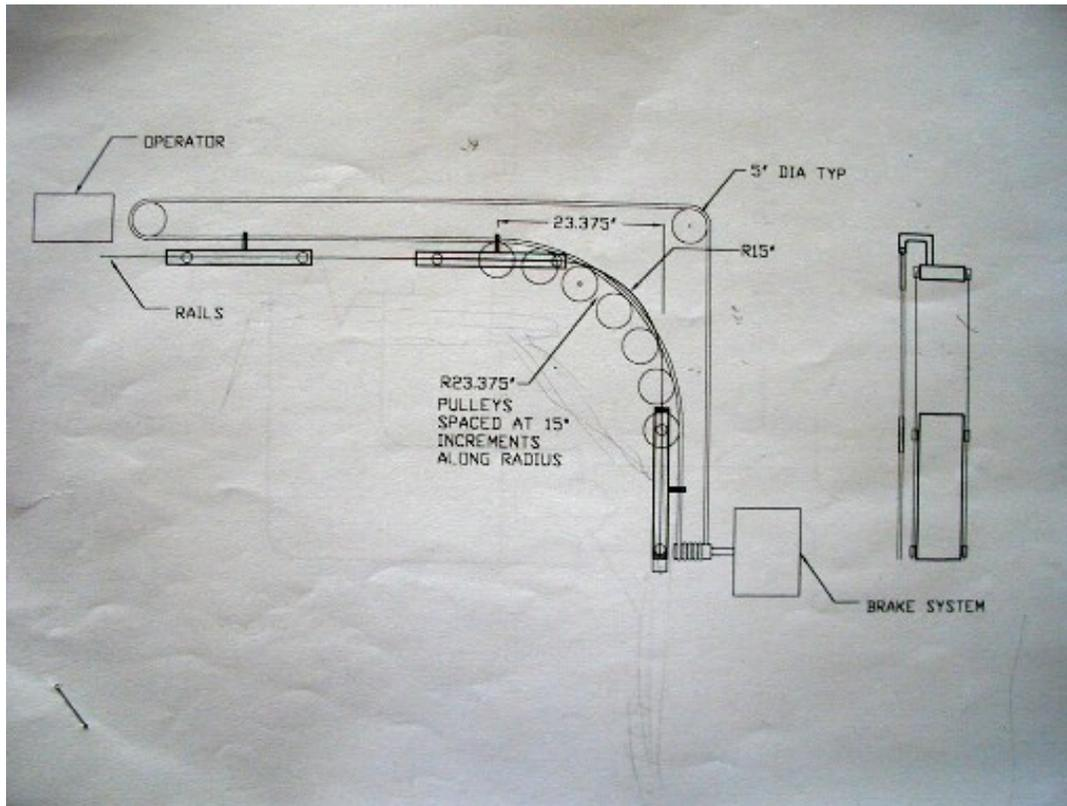
Our third and final design was much simpler. A second chain-driven rail, a standard garage door operator part, was attached to the frame above the first rail. Two arms attached this rail to the door panel. The sprocket at the end of this second chain is coupled to an electric brake. This design allows us to apply friction loads to the arm while using existing parts from Chamberlain. The simplicity of this design is one of its greatest strong points.
