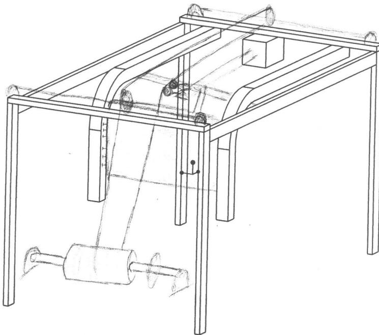
The next design was the first to implement a brake. This design has a ski-lift arm attached to the door. This arm is connected to a cable that runs parallel to the path of the door, along a system of
