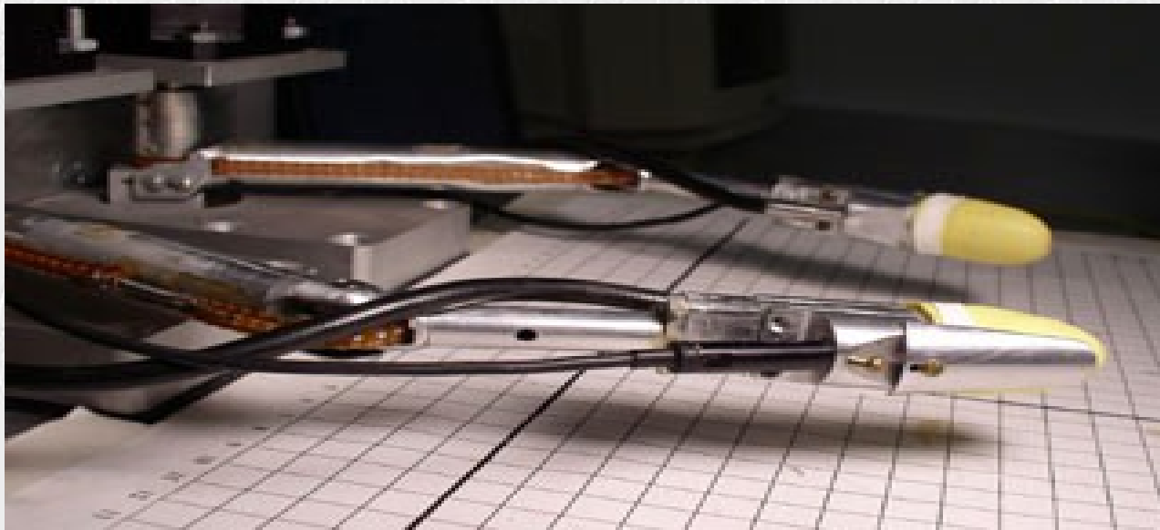
The HRL Manipulator at Harvard University, which has sensors, attached.
