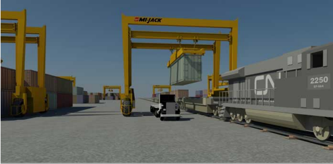
Fig. 4-x. Mi-jack Gantry Crane Lifts Container Off Train And Prepares To Load Truck.
