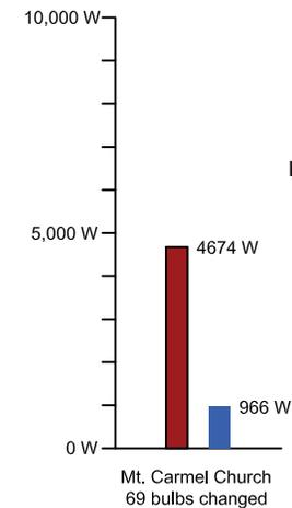
In Mount Carmel church, we replaced 69 light bulbs ranging from 60 to 300 watts with new, longer lasting 14watt bulbs. This change will save the church 3708 watts per hour, which translates to approximately \$1158.75 off their electricity bill per year.
