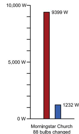
In Morningstar church, we replaced 88 light bulbs ranging from 60 to 300 watts with new, longer lasting 14watt bulbs. This change will save the church 8168 watts per hour, which translates to approximately \$1020 off their electricity bill per year based on the church's use.
