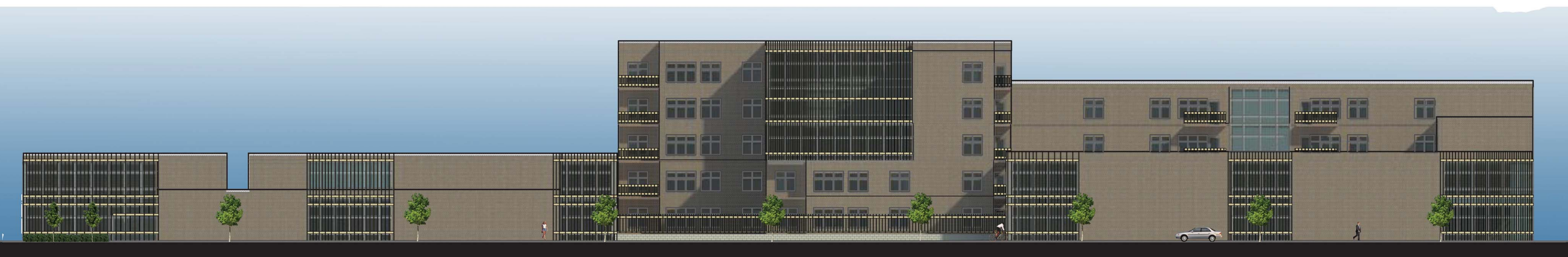
South Elevation: showing brick facade with wood screens
