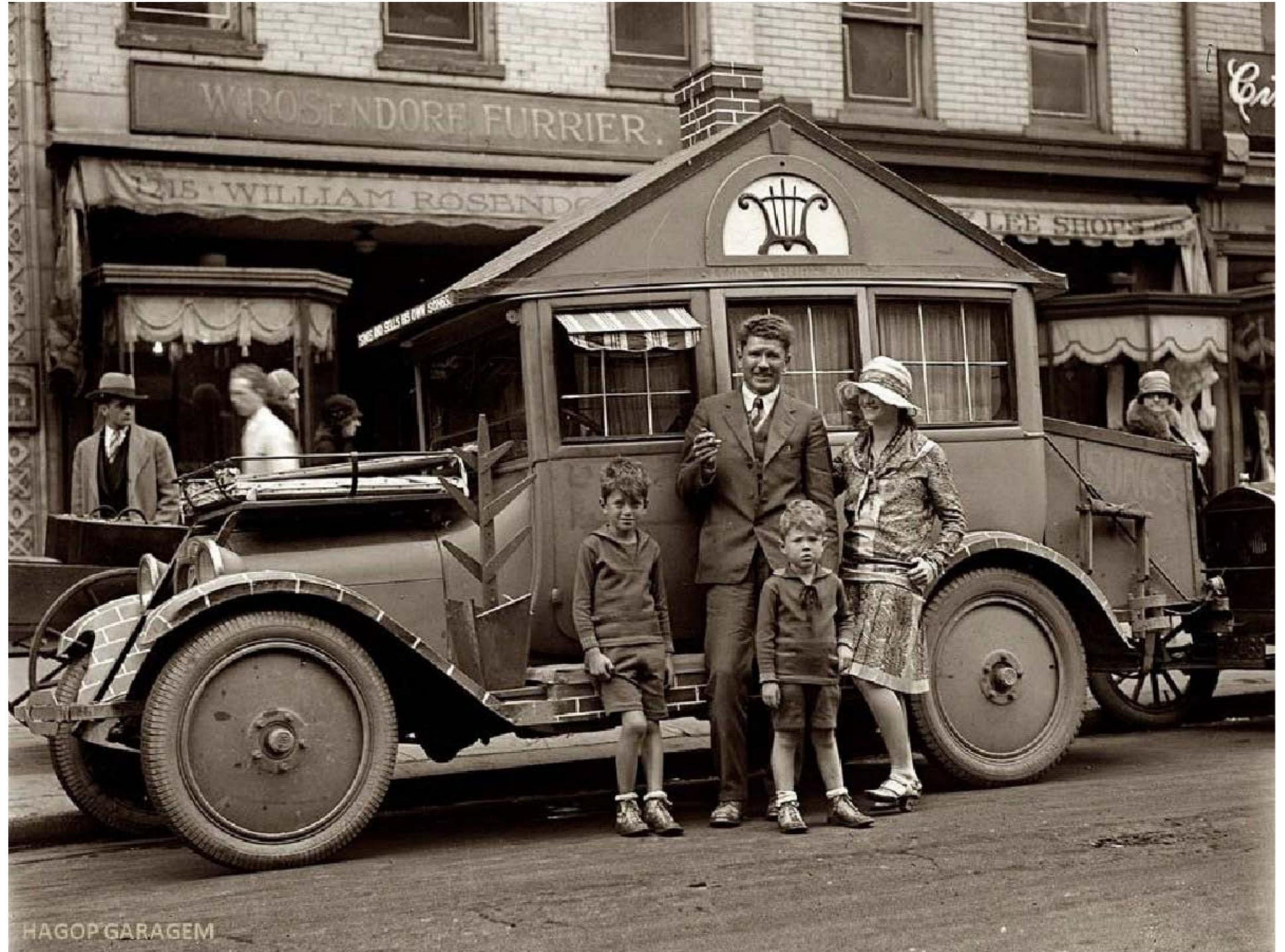
The Thompson House-Car was built in 1934 intended for trips in the African Safari. It was known for its telescoping roof. When extended it expanded the interior space of the vehicle, and when retracted it improved the efficiency output of the vehicle while driving.
