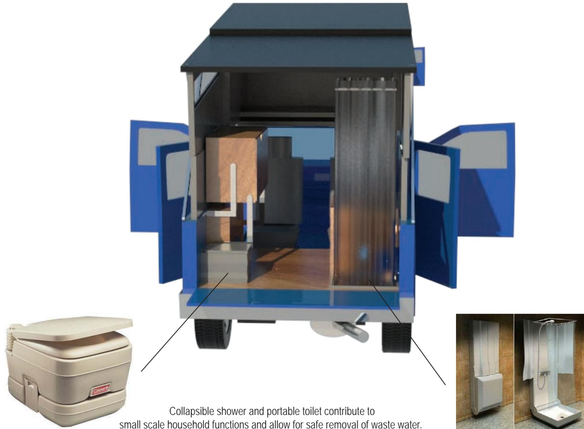
Collapsible shower and portable toilet contribute to small scale household functions and allow for safe removal of waste water.
