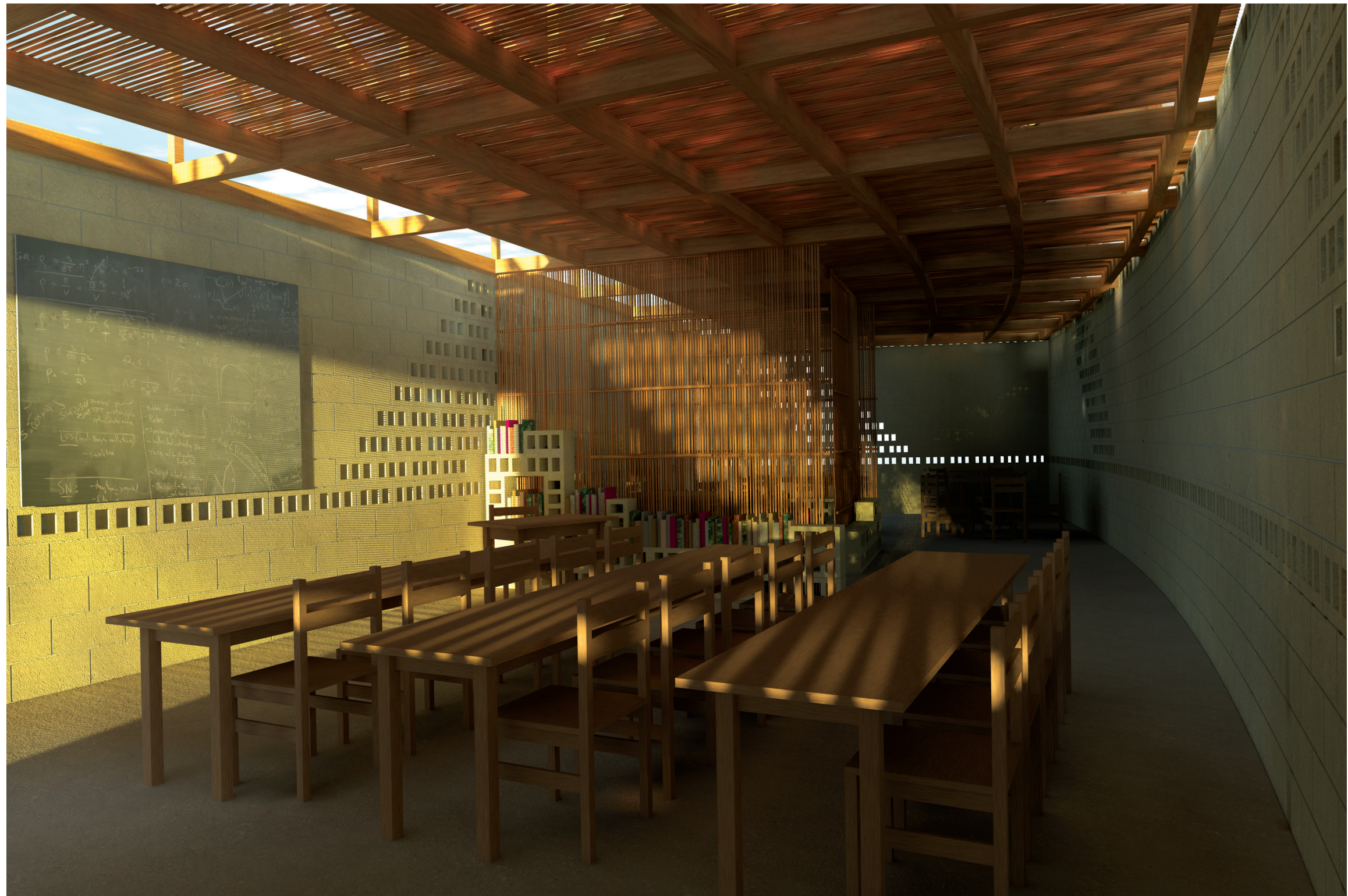
The horizontal band of block at eye level brings in light and allows the children to view the site from their own vantage point. It also provides a benchmark against which the children can measure their own development. The height of the lower horizontal band will be determined by the height of the students in the studio; the secondary and vocational schools would have a higher band to match the eye level of taller children. Over the course of their education, students will be able to measure their physical growth by identifying the CMU course through which they can see outside. The larger block openings will remain constant, always providing the children with a sense of growth and progress.
