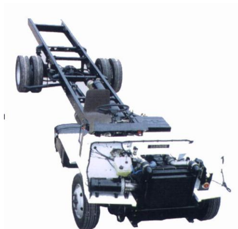
Figure 23 – Example of a typical bus chassis showing frame construction
