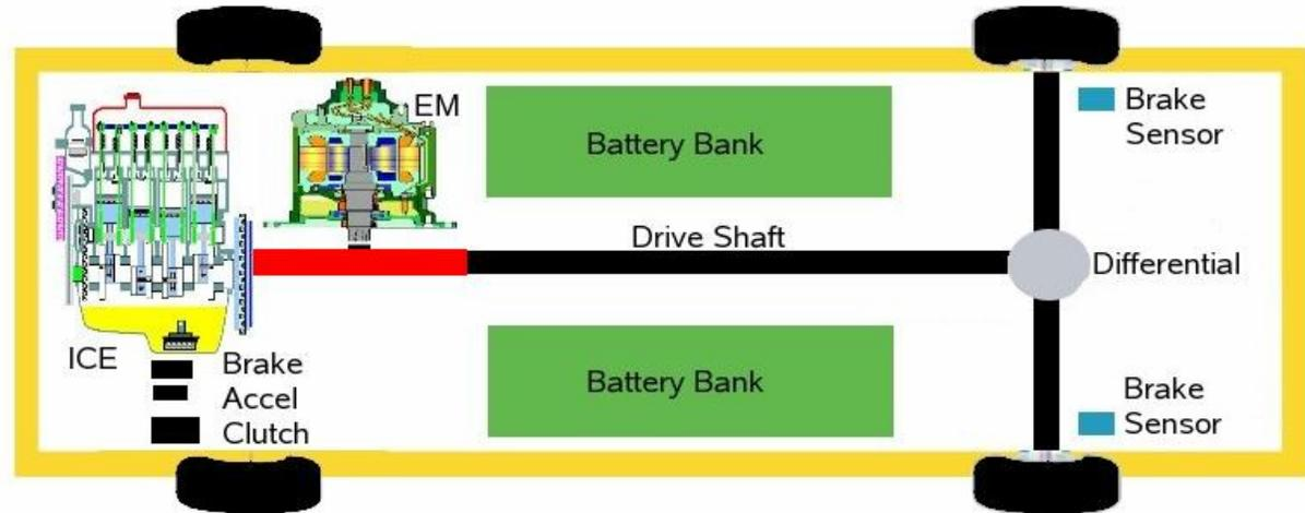
**RC Model Car:** demonstrates the hybrid concept on a very small scale. A typical model car using an internal combustion engine was modified to incorporate an electric motor. The model thereby employs a combined ICE/EM system to improve performance by increasing the total vehicle power and improving the instantaneous acceleration.
